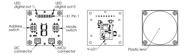
The V-LD1 evaluation kit consists of an evaluation kit PCB with a mounted V-LD1 in combination with a plastic lens which is mounted per default. The kit contains an FTDI cable which can be connected directly on connector X1 to power the sensor and create a virtual COM port connection to the PC.
