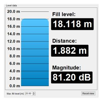
This view shows the measured distance and magnitude in real-time and provides the option to visualize it as a fill level of e.g. a tank.
