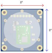
The lens can focus the beam width to about  $8 \times 8$  degrees and has a typical gain of 12 dBi. It is possible to integrate such a lens directly into the housing of a final product.
