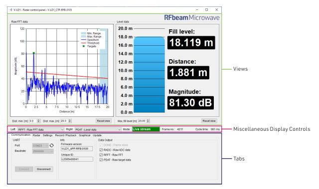
There are many views to select in the miscellaneous display controls area. All of them have a preceded shortcut based on the data output which is used in the views (RADC, RFFT, PDAT). To use the different views the according data output needs to be enabled.
