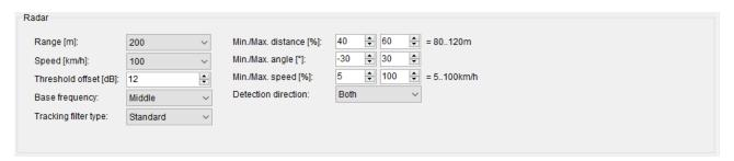
This tab controls the main settings of the processing chain in the radar sensor. By changing these parameters, it is very easy to adapt the sensor to the needs of an application and check the influences in real time. A detailed description of all parameters can be found in the chapters Radar Settings and Detection settings of the K-MD7 datasheet.
