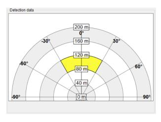
The sensor features a customisable detection zone filter to signal a detection on digital output 0 if in minimum one TDAT target is inside of the defined yellow detection zone.
