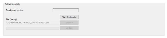
This tab allows the update of the K-MD7 firmware over the se $rial\ interface.\ The\ sensor\ starts\ to\ the\ application\ per\ default.$ The «Start Bootloader» button gives the option to start the  $bootloader\,out\,of\,the\,application.$
