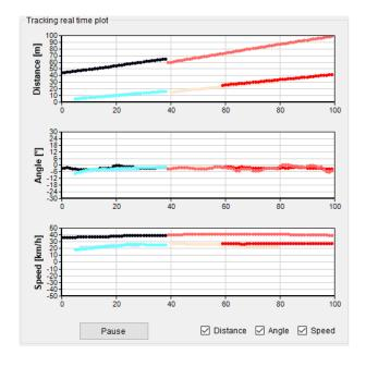
This view is very helpful to analyse the tracked targets. It visualises the distance, angle and speed over the time.
