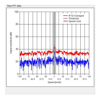
The RFFT view shows the average frequency spectrum of the two receiving channels. Further the threshold is visualised. Each movement which generates a frequency with an amplitude above the threshold is used for the calculation of the raw targets.
