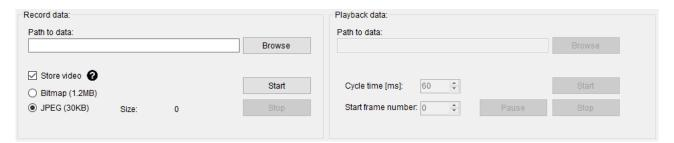
This tab can be used to record and playback the sensor data to the hard disk. It is also possible to store the video data in parallel what can be helpful to interpret the measured data in the playback mode.
