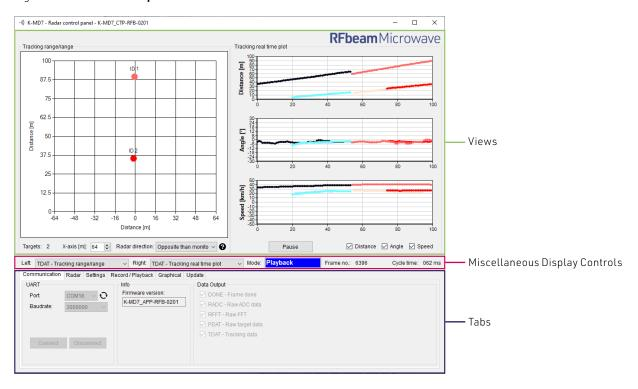
There are many views to select in the miscellaneous display controls area. All of them have a preceded shortcut based on the data output which is used in the views (RADC, RFFT, PDAT, TDAT). To use the different views the according data output needs to be enabled.
