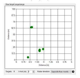
This is one of the most interesting views, as the information of the targets is interpreted and shown in a two-dimensional map. The targets show the radar's view of the real world and colours the points according to the direction of the movement. It is possible to change the scaling of the X-axis.
