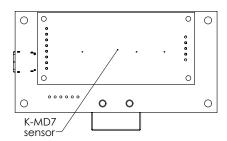
The K-MD7 evaluation kit consists of an evaluation kit PCB in combination with a tripod mount and a K-MD7 sensor. There is an USB-C connector mounted on the PCB for powering and connection the K-MD7 directly to a PC. Further there is a detection LED mounted on the board to visualise if the sensor has detected any targets inside of a definable zone.
