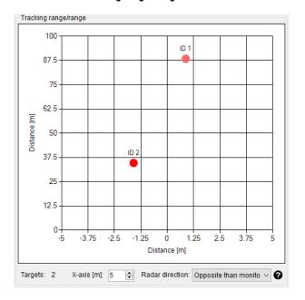
Compare this view with the corresponding raw view (PDAT) to see the improvements of the tracking filter. It is possible to change the scaling of the X-axis.
