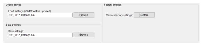
The settings tab features the possibility to easily save and reload the complete settings of a sensor. This makes it easy to duplicate a useful dataset to multiple sensors. Further it is possible to restore the default factory settings.
