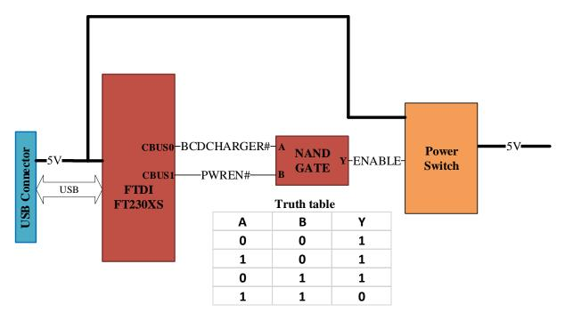
Figure 2. Block Diagram showing the logic control of the Power Switch ENABLE signal.
