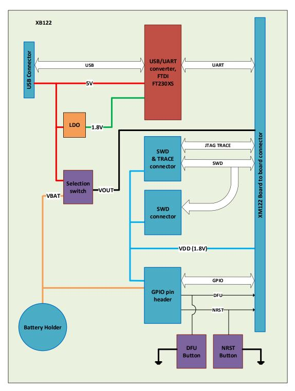
Figure 1. The block diagram of XB122.
