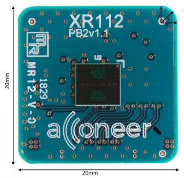
x=y=2.05mm r = 2.9mm PCB thickness: 0.9mm
