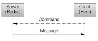
The communication is based on a client-server model. There are two types of packets transmitted. Commands are sent from client to server and messages are sent from server to client.
