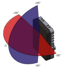
The angle is calculated in degrees and is valid between  $\pm 86^{\circ}$ . If an object has an angle of zero in azimuth and elevation, it is directly in front of the sensor.
