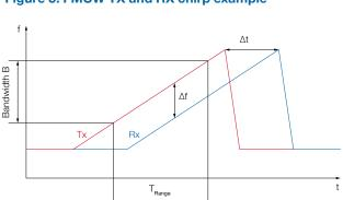
the reflected signal is demodulated and sampled by the ADC for each RX antenna. Objects with different distances thus generate different frequencies in the sampled time domain signal. An FFT is used to transform the ADC samples into the frequency domain. The FFT magnitude spectrum contains the reflections of all objects in front of the sensor, which are represented by different frequencies. The higher the frequency, the further away the object is.
