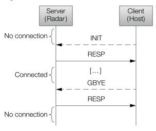
To connect and disconnect from the radar module a connection procedure is used. The client has to send the INIT command over TCP/IP to establish a connection with the server. To disconnect from server the GBYE command must be sent from client.
