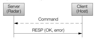
Every command sent by the client is acknowledged by the server with a response message (RESP). The response message includes information data about the success or failure of the received command.
